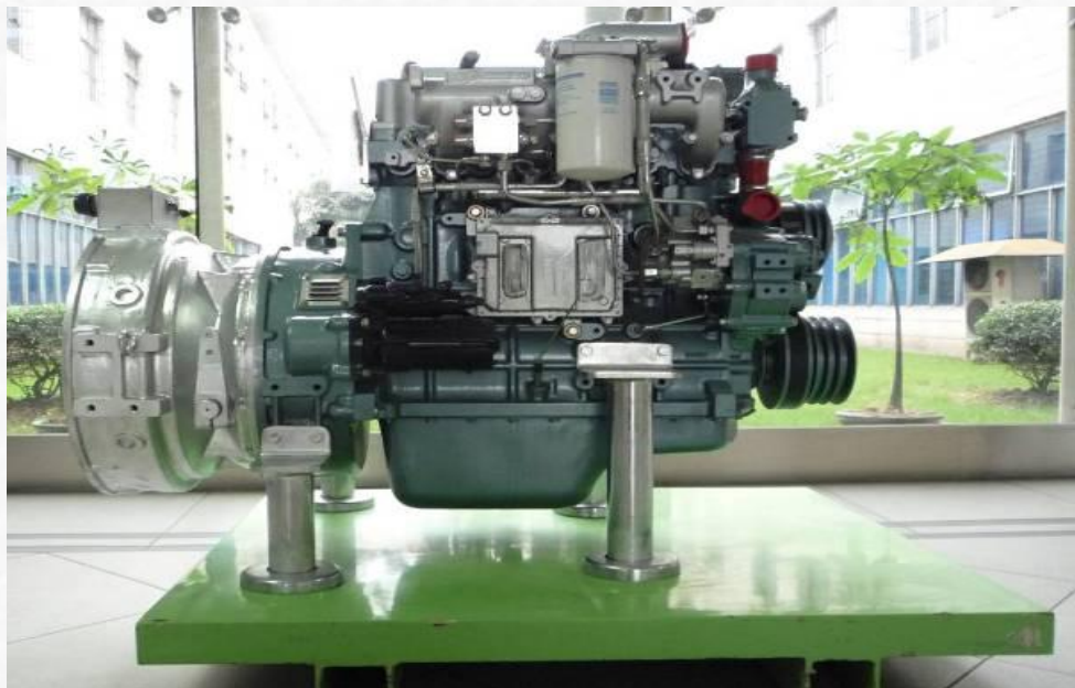
Yuchai engine coupled to Electric Motor Drive
