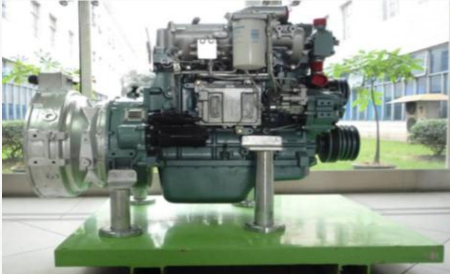
Yuchai engine coupled to Electric Motor Drive
