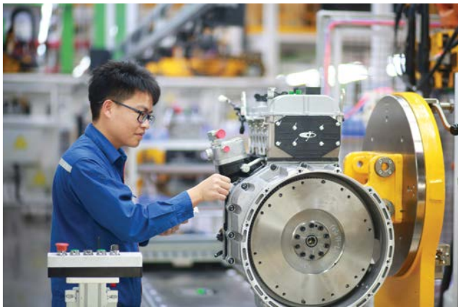
A worker on the assembly line is attaching QR code with ID information on the engines.
