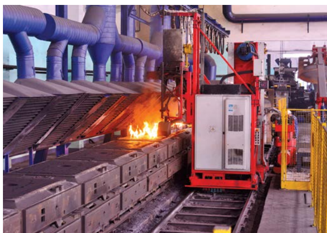
Yuchai's cylinder head foundry molten iron auto-feeding system
